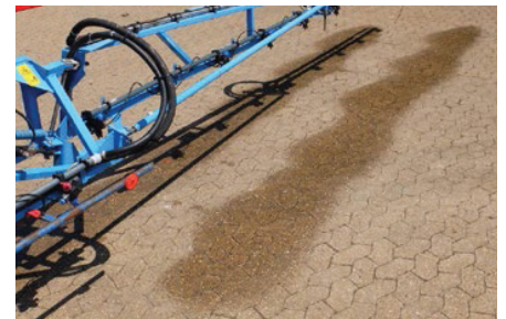
Designed to ensure even spray distribution on both sides of the boom when the nozzles are installed in alternating directions
