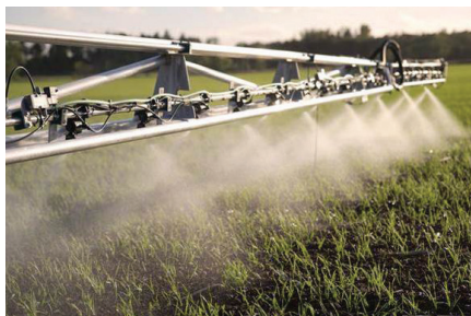
Install facing in alternating directions along the boom to provide coverage on both sides of the target
